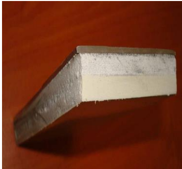
Steel Tank Lining Sample
