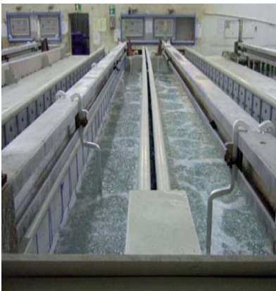
TANK LININGS WITH PP
