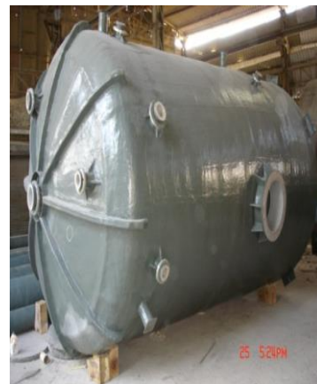
PVDF FRP 20M3 Chlorate Tank
