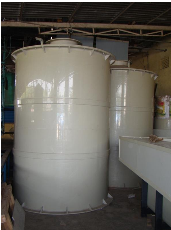
PP (Polypropylene) 50M3 ACID TANKS
